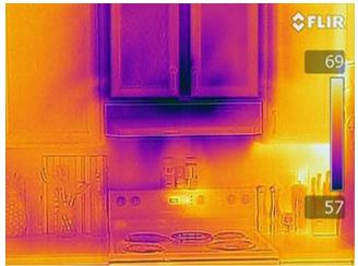
Cold air infiltration from the exhaust duct.
