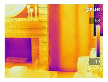
Missing and displaced insulation. *Invisible to the naked eye*.
