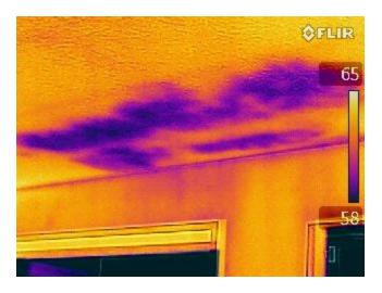
Water leak. *Invisible to the naked eye.*
