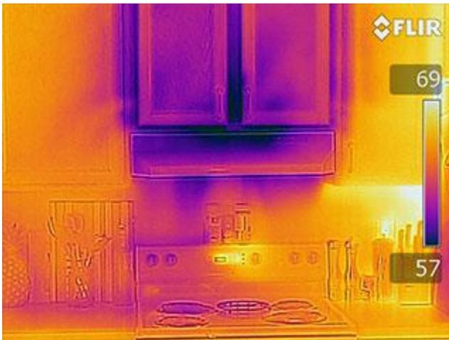
Cold air infiltration from the exhaust duct.
