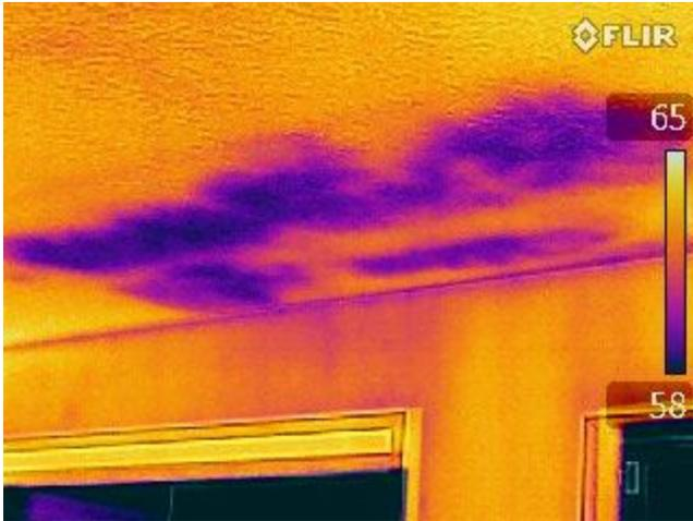
Water leak. *Invisible to the naked eye.*
